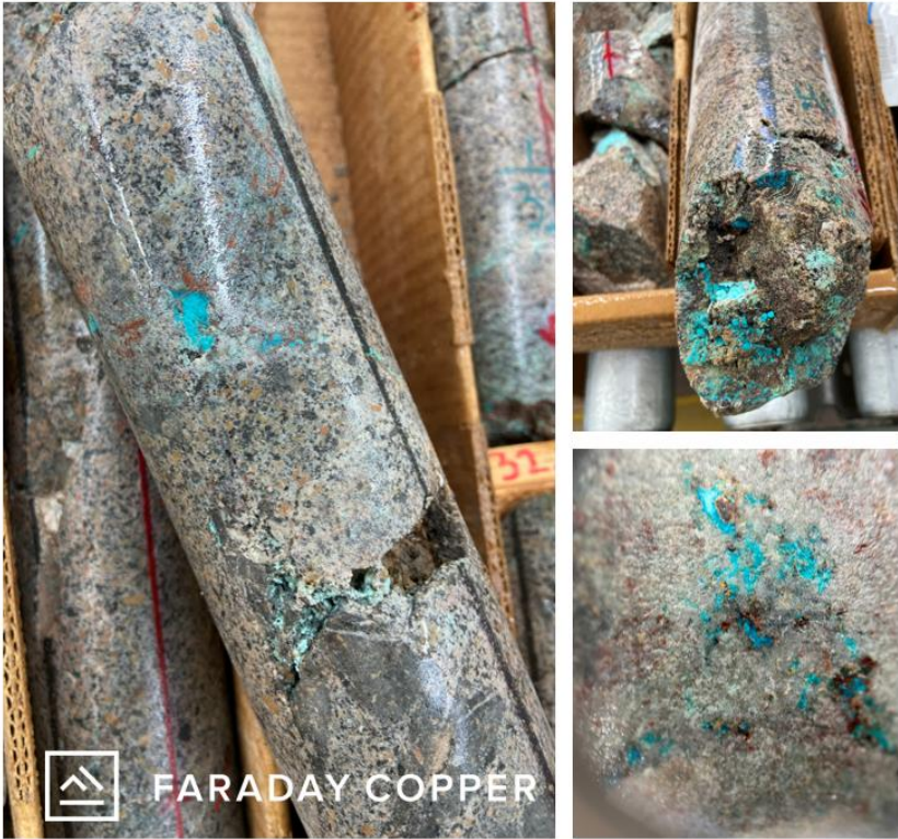
Figure 3: Images of Copper Oxide in Turquoise Color (chrysocolla) Present in Core from Drill Hole FCD-26-173
