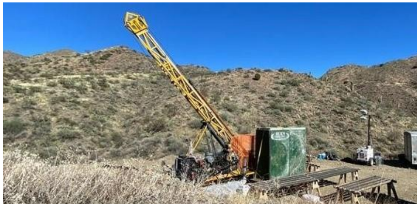
Figure 1: Diamond drilling in Hole #3
