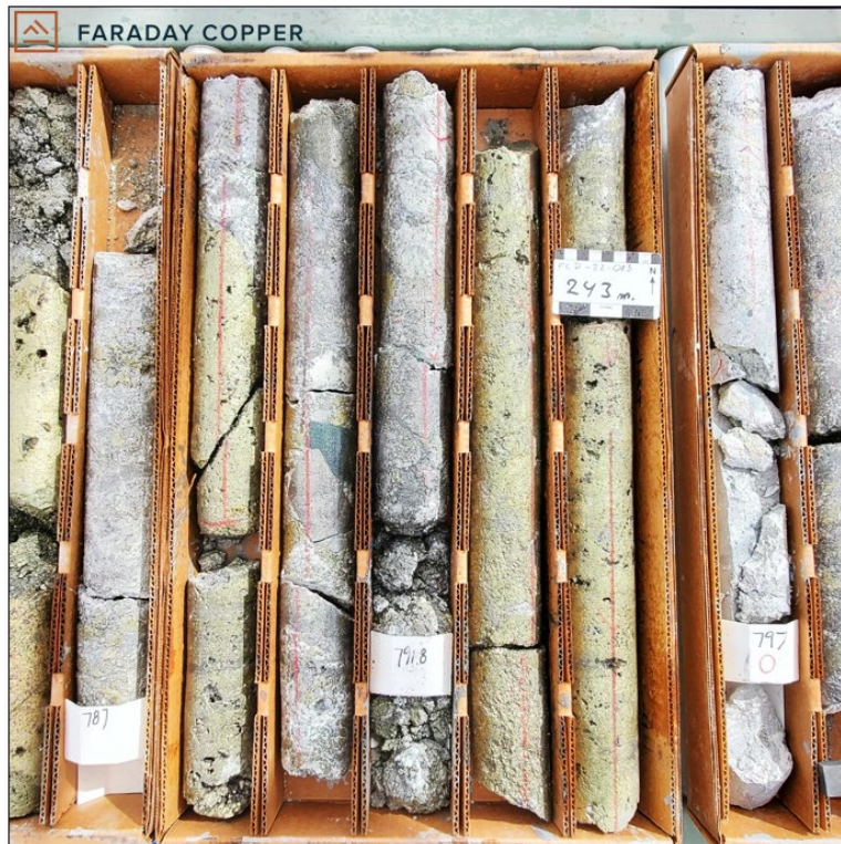
Figure 1: A portion of drill core from Phase II drill hole FCD-22-013 showing massive copper sulphide from the Copper Prince breccia at the Copper Creek Project ( assay results are pending )
