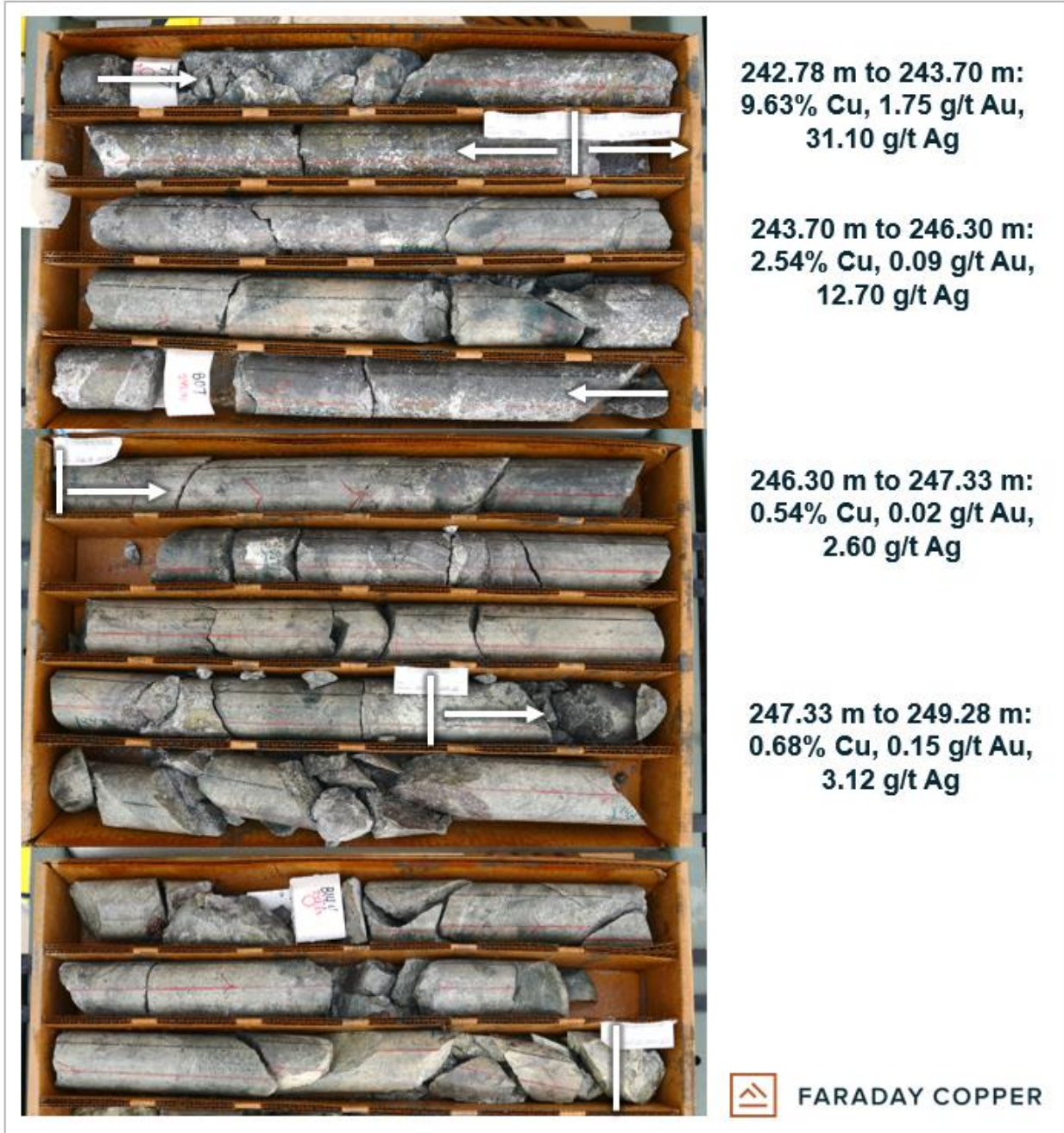
Figure 4: Photographs of the High-Grade Mineralization in Drill Hole FCD-22-013 (242.78 m to 249.28 m) at Copper Creek
