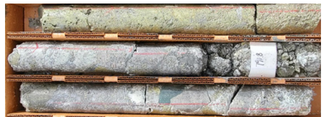
Hydrothermal breccia containing massive sulphide from drill hole FCD-22-013 at the Copper Prince breccia, which intercepted 15 metres at 10.83% copper, 1.65 g/t gold and 55.62 g/t silver 3
