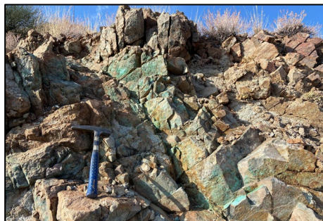
Near resource target: Copper oxide mineralization exposed at the Hilltop breccia target
