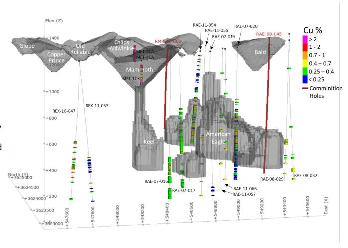
Notes: The image displays metallurgical composite samples overlaid with open pit shells (based on 0.23% cut-off grade) and underground shapes (based on 0.31% cut-off grade) used to constraint the MRE.
