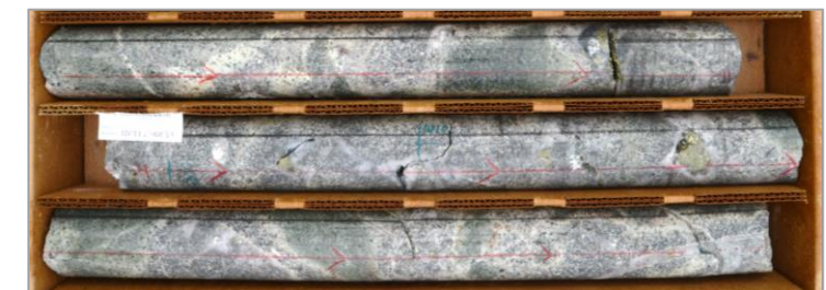
Core from mineralized breccia of drill hole FCD-23-024
