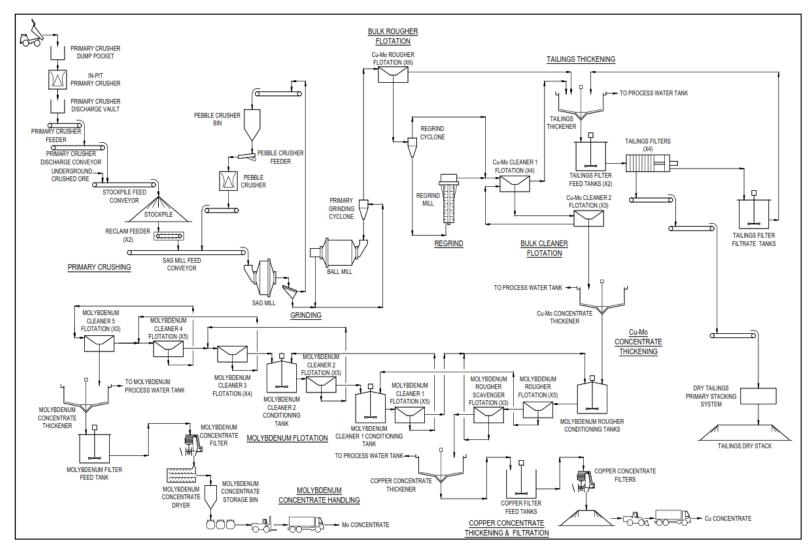
Figure 17-1: Concentrator Flow Diagram for Sulphide & Transitional Materials
