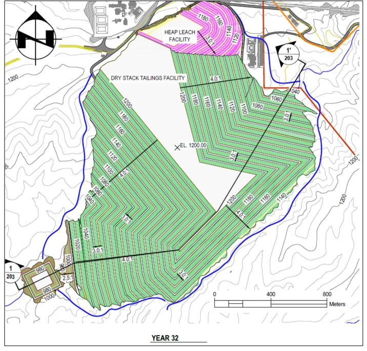
Figure 18-7: Dry Stack Tailings Facility Arrangement Year 32
