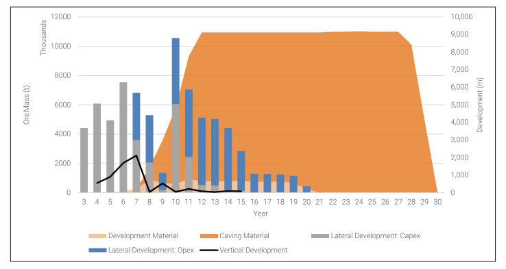
Figure 16-35: Underground LOM Schedule; Development Metres and Mineralized Material Tonnes
