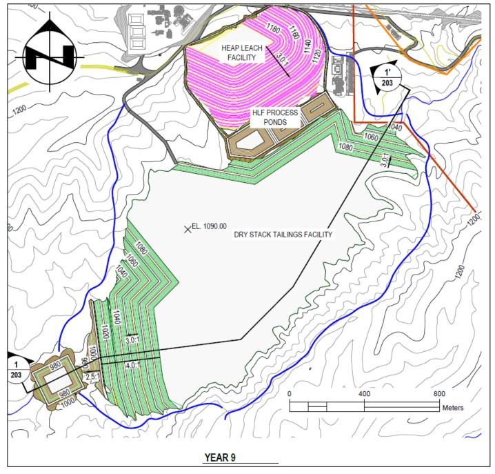
Figure 18-6: Dry Stack Tailings Facility Arrangement Year 9
