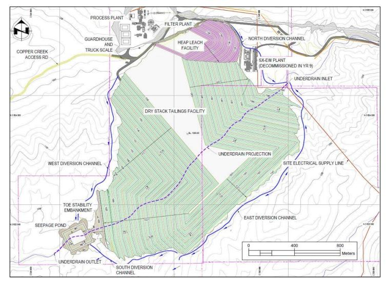
Figure 18-4: Ultimate Dry Stack Tailings Facility General Arrangement
